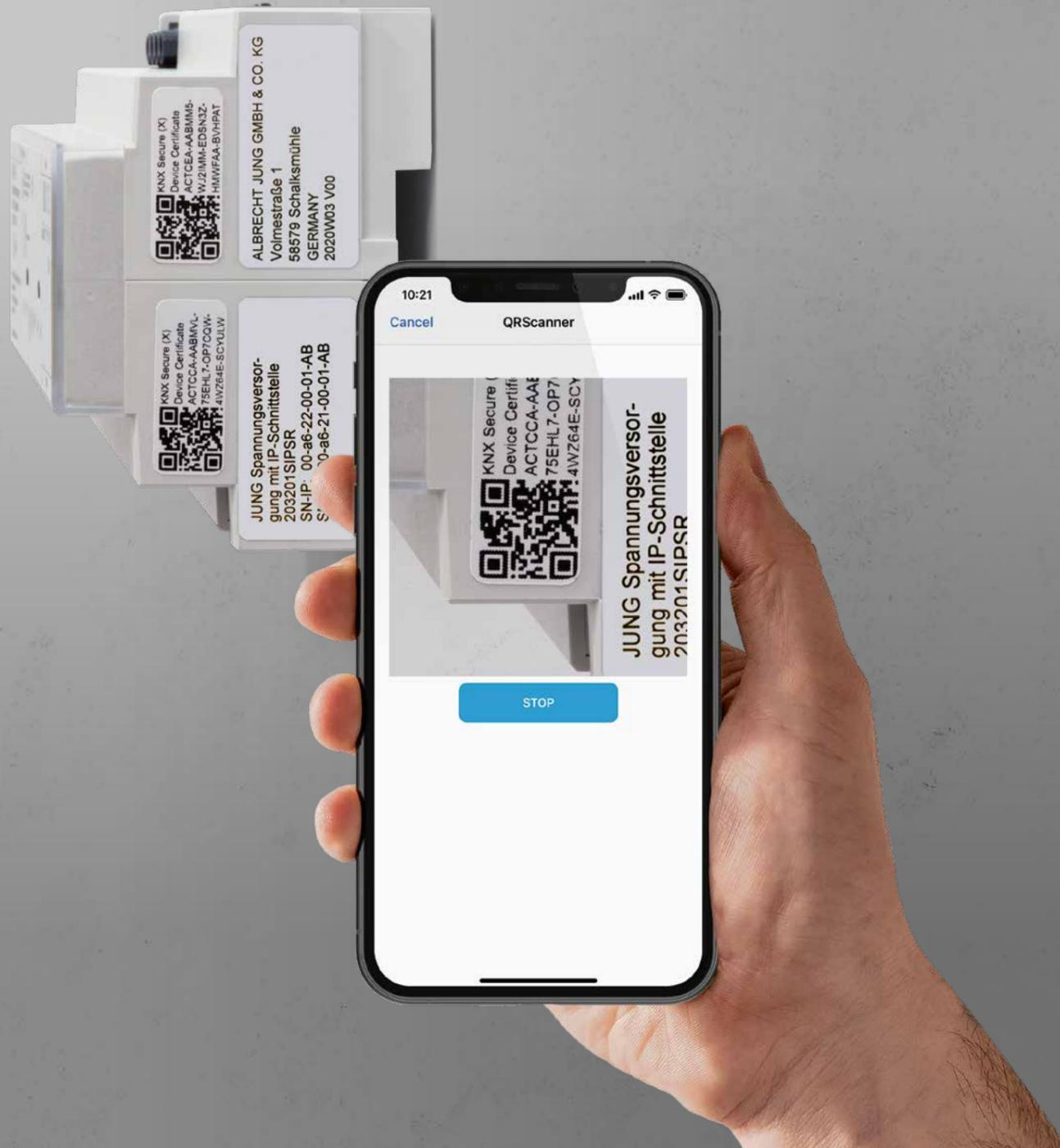
Professional installers need the certificates of the individual KNX Secure components to make a KNX installation secure. They are printed on the devices as a QR code and must be integrated into the ETS. The easiest way to do this is via app.
