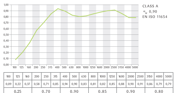
Example: sound absorption coefficient for PLANLICHT p.quiet with Organoid® absorber in the one-third bands and octave middle frequencies
